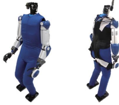
Fig. 2. Overview of humanoid robot HRP-4 (Left). The robot can wear the human assistive device (Right).
