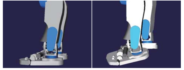
Fig. 3. Initial feet posture in the retargeted motions. The left and right figures show the results with and without constraint respectively.
