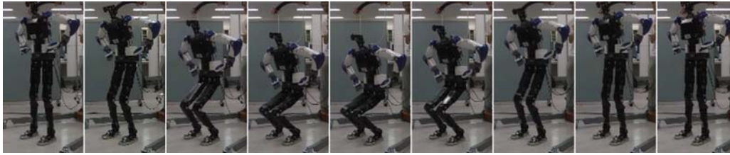
Fig. 6. Experimental result of retargeted squat motion using smoothing with stability constraints with humanoid robot HRP-4
