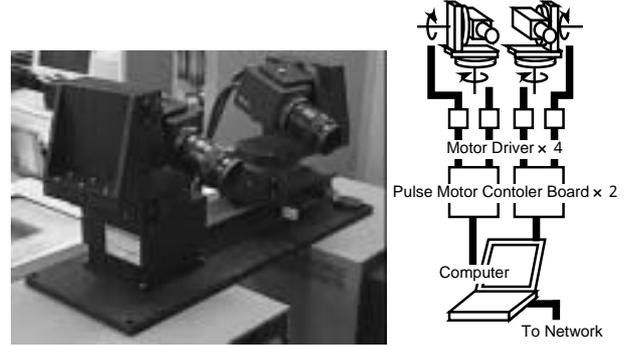
Figure 4: Stereo camera system.
