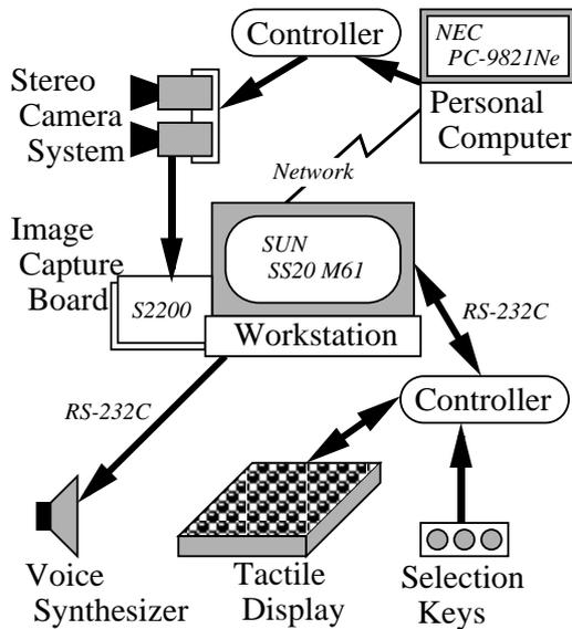
Figure 3: Composition of the interactive tactile display system.
