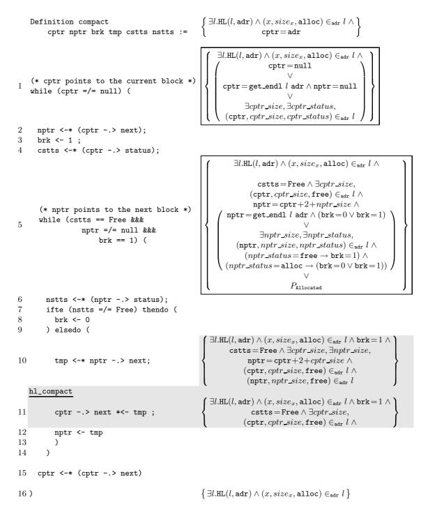
Fig. 4. Proof sketch of compact (partial proof of hmAlloc in Fig. 2)
