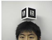
Figure 6. The visual marker for the AR toolkit method.
