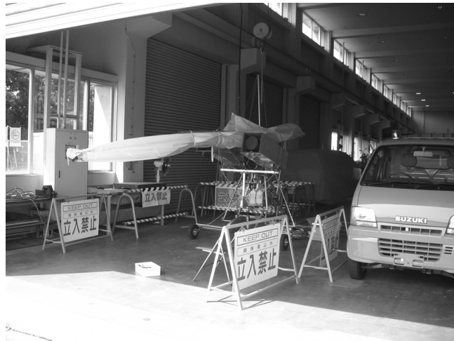
Fig. 11 The folded 3DTR-I can only occupies a small parking surface area.
