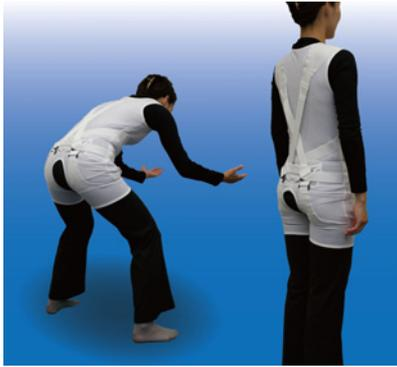
Fig. 2: Assistive wear “Smart Suite Lite (SSL)”
