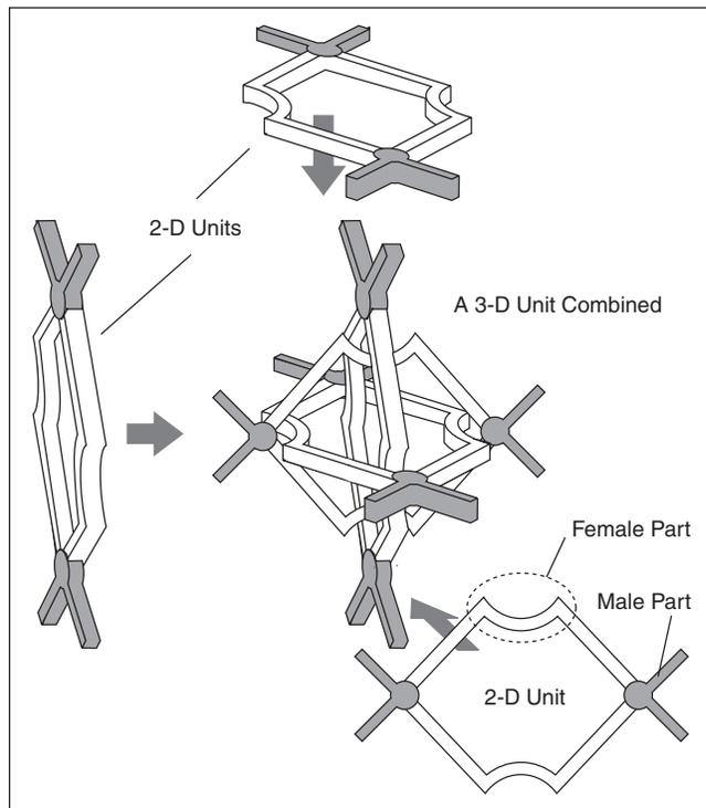
Figure 14. A 3-D module composed of three 2-D SMA modules.
