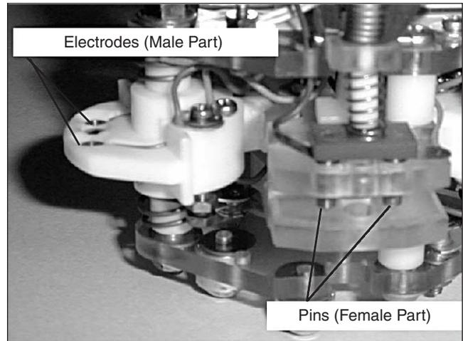
Figure 8. Intermodule connection for communication.
