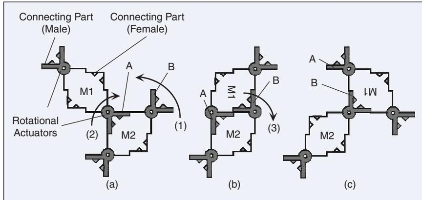
Figure 2. "Step motion" of two modules.
