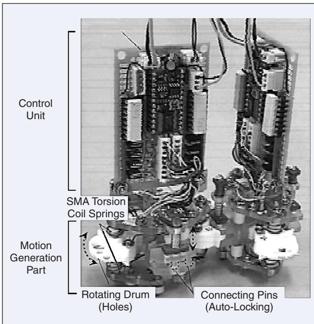
Figure 6. Overview of prototype module (First model).
