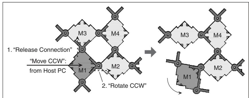
Figure 9. Local motion coordination through intermodule communication.
