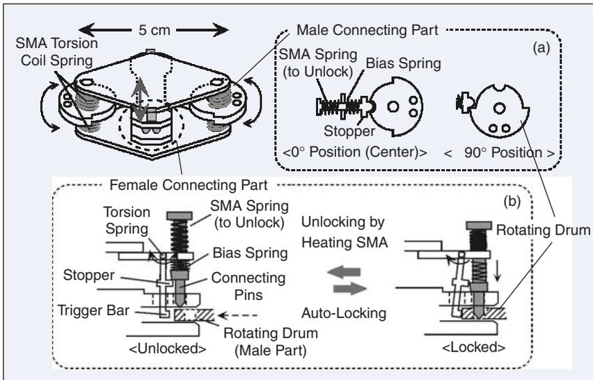
Figure 5. Structure of the prototype module.
