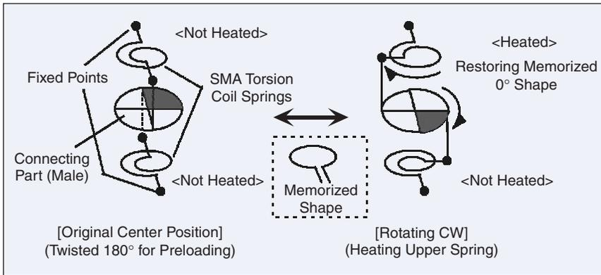
Figure 4. Rotating actuator mechanism using SMA torsion coil springs.
