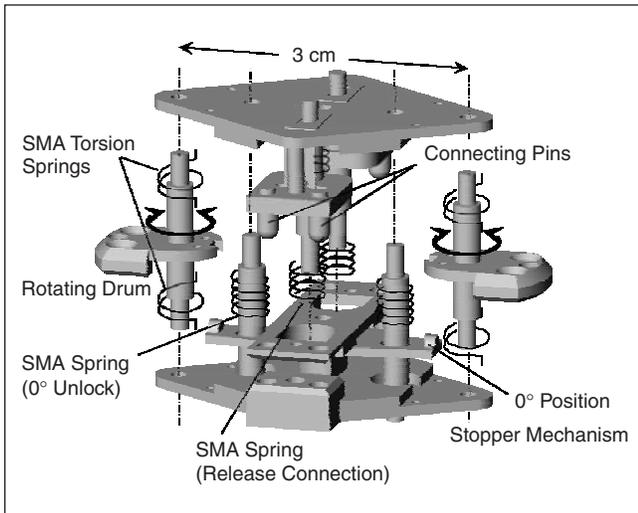
Figure 11. Structure of micromodule (second model).
