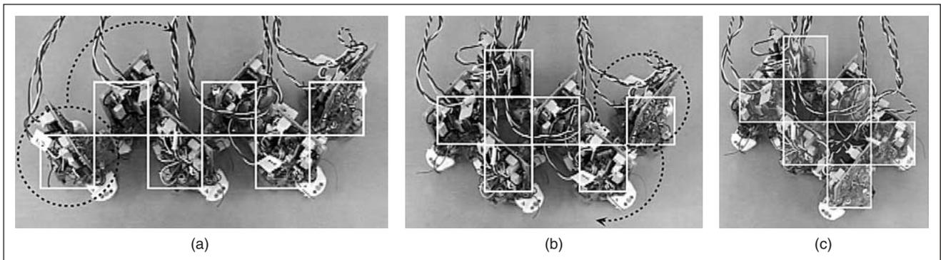
Figure 10. Self-reconfiguration experiment using six modules. (a) Initial state. (b) Transient state. (c) Self-reconfiguration completed.
