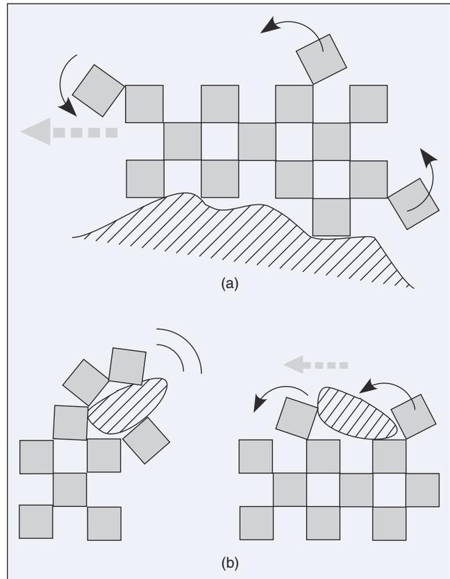
Figure 3. Various shapes and movements generated by self-reconfigurable modules. (a) Moving. (b) Handling and transporting an object (with fine control of SMA).
