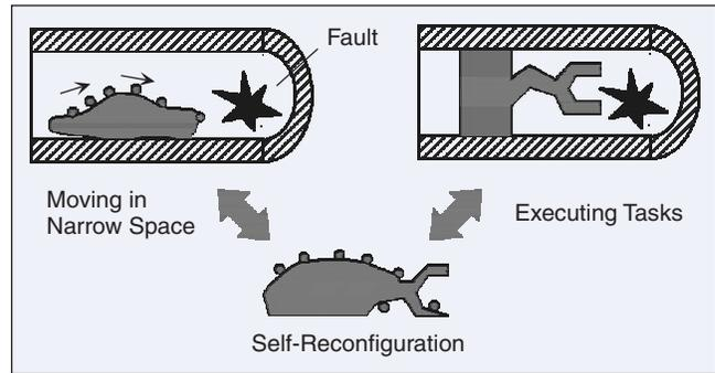
Figure 1. Applications of a micro self-reconfigurable robotic system.
