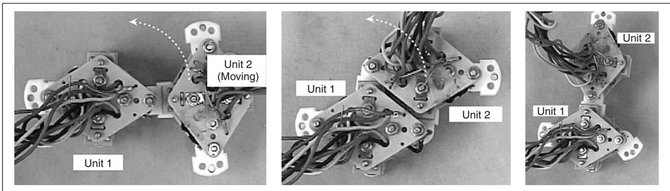
Figure 13. Experiment of basic motion by two microsize modules.
