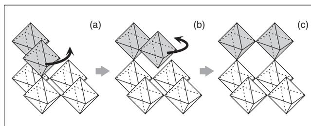
Figure 16. Motion of 3-D SMA modules.
