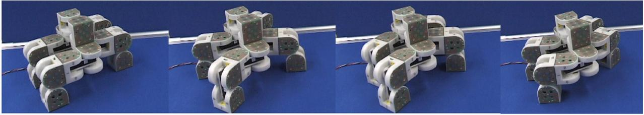
Figure 11: Motion of the quadruped robot (Type 1)
