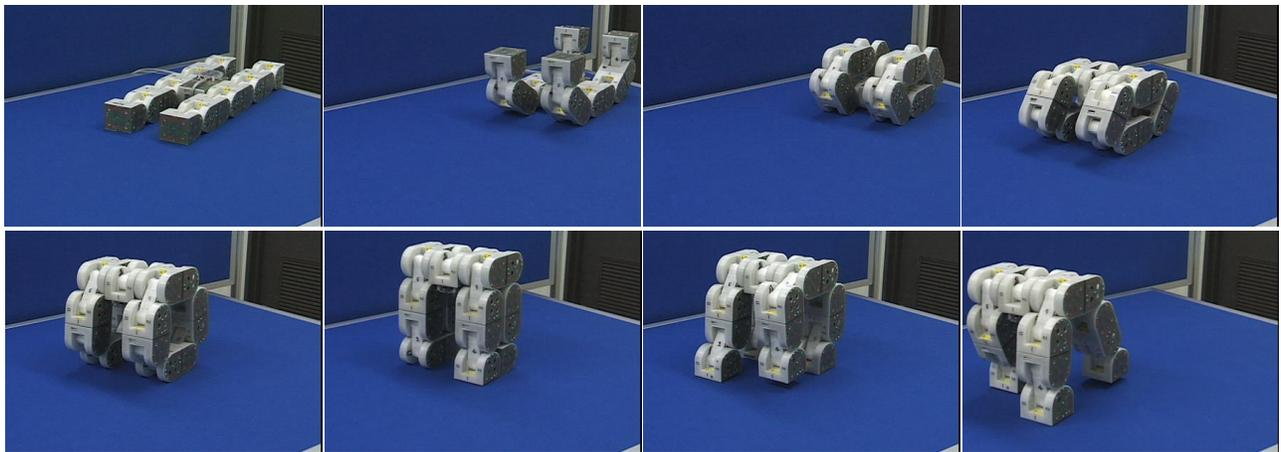
Figure 14: Transformation of the crawler to the quadruped robot (Type 3)
