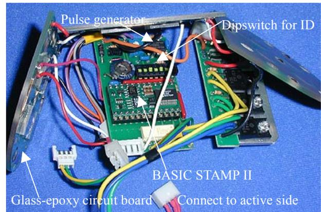
Figure 5: Control circuits in the passive side
