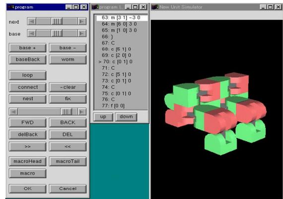
Figure 9: Screen capture of the developed simulator
