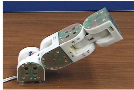
Figure 4: Lifting up motion with two modules
