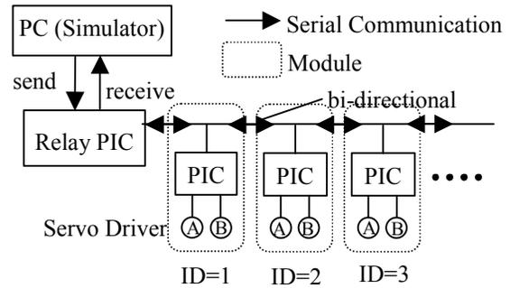
Figure 7: Schematic of the control system architecture
