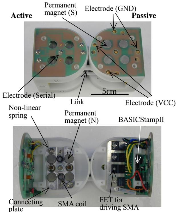
Figure 3: Photos of appearance and inner structure of the developed module
