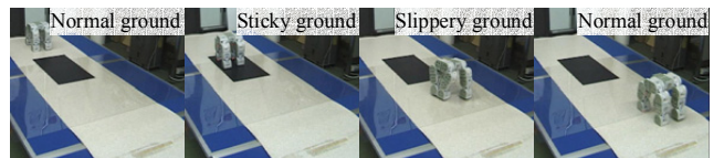
Figure 15. Adaptation to normal, sticky and slippery ground by 4-legged robot.
