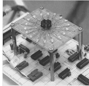
Fig. 18 Photo of infrared communication device.
