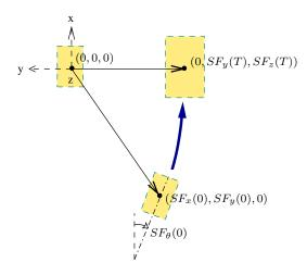
Fig. 1. Here we show an upward half-step from above. It is fully determined by the 5 parameters  $SF_x(0)$ ,  $SF_y(0)$ ,  $SF_\theta(0)$ ,  $SF_y(T)$  and  $SF_z(T)$ . A downward half-step is also fully determined by 5 parameters.
