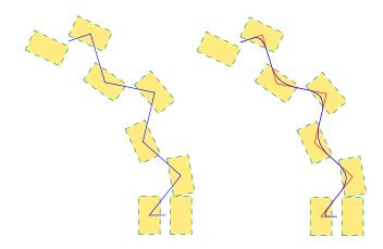
Fig. 4. We illustrate the "smoothing" of a raw sequence of half-steps. On the initial raw sequence (on the left) we can see that the support paths for the ZMP and CoM trajectories are superimposed. Then, after adjusting the overlaps, the ZMP support path stays the same but the CoM support path becomes smoother (on the right, ZMP in red and CoM in blue).
