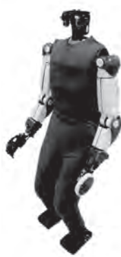
Fig. 2. HRP-4 with a soft body surface.
