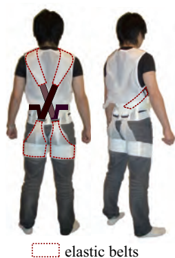
Fig. 1. Passive power-assist device "Smart Suite Lite".
