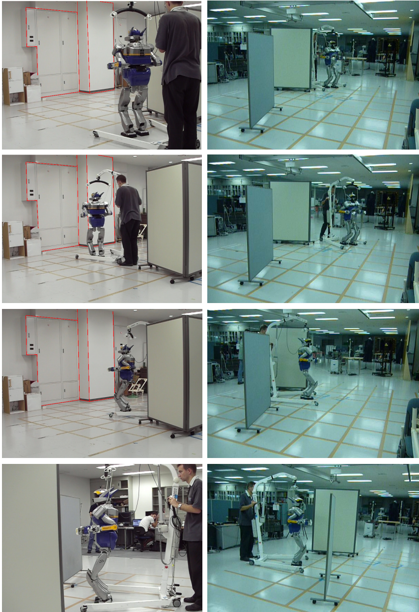
Fig. 11. The execution of a trajectory with obstacles on the HRP-2 robot at four time stamps, from two different points of view.
