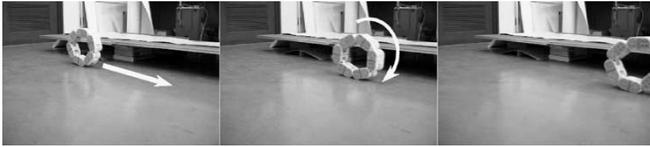
Fig. 19. Snapshots of rolling motion by the crawler configuration [Fig. 6(d)]. Rolling motion was successfully realized by the real-time CPG control.
