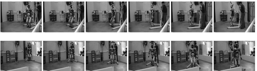
Figure 8. Experimental validation of optimal paths on the HRP-2 robot (test cases 2 and 6).
